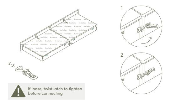
Hook storage box stopper underneath front rail.
