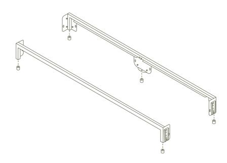
**9** Slide centre beam into slot on front and back rail.
