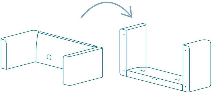
**3.** Screw baseboard with the velcro facing in, onto frame using the longer length thread legs in the order shown.
