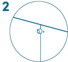
**6.** Screw baseboard to frame using the longer thread length legs in remaining positions.
