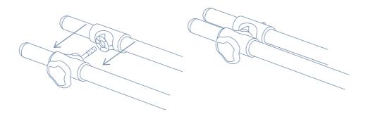
Using the non-threaded gumnut, screw it onto the visible thread. Do not tighten fully.
