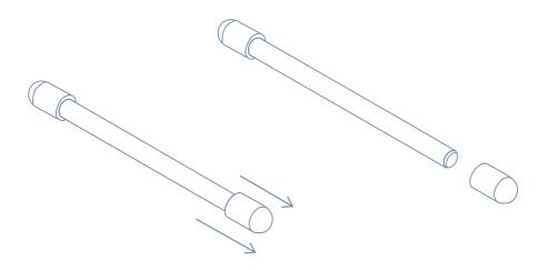
Slide the leg through the T-joint and re-attach the end cap on the other side. Repeat for both legs.
