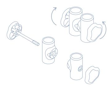
Take one hinge and slide it over the top of the tent pole so that the holes align and then put the thread of the gumnut through the hole.
