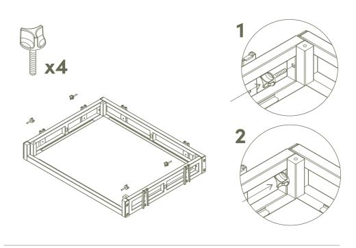
Screw on the legs with washers until fully tightened.
