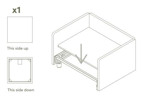
Align and push in the storage box under the front metal beam.
