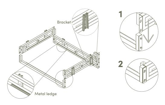
2. Ensure the metal frames are flush with each other before moving to the next step.
