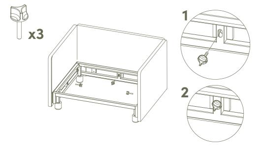
Place the seat base frame onto the metal ledges on the metal frame.
