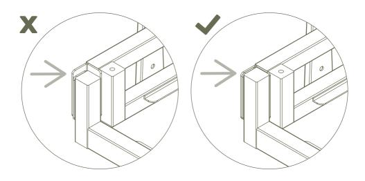
Lock the metal frame together by inserting gumnuts x4 into the corners as shown, and tighten fully.
