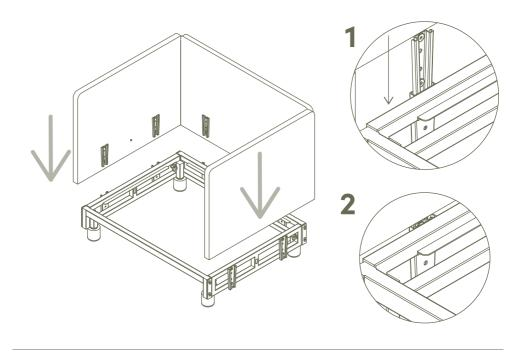
6. Insert the gumnuts through the metal frame into the armrests and backrest and tighten fully.
