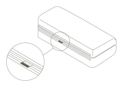
**27.** Place Seat cushion on top of cover so that tab colors are matching. Secure the velcro on the front and rear of the Seat cushion.
